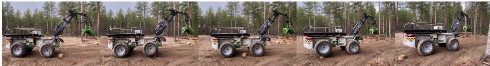
Figure 6: SAHA-2 with active chassis control driving over a tree trunk with its right wheels. The active chassis balancing ensures contact of each wheel during the process.
