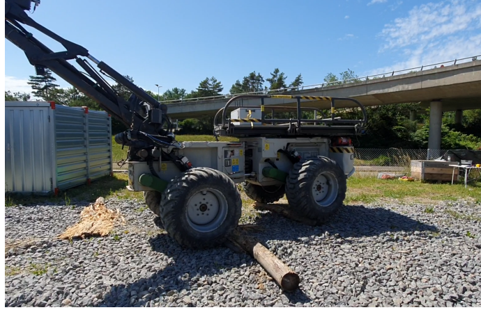
Figure 3: Experiment of SAHA driving over logs.
