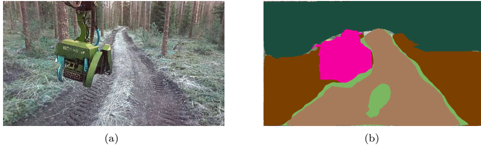
Figure 2: Semantic-based terrain segmentation on RGB camera image input. a) shows the raw RGB camera input. b) shows the semantic segmentation for different reversibility classes.
