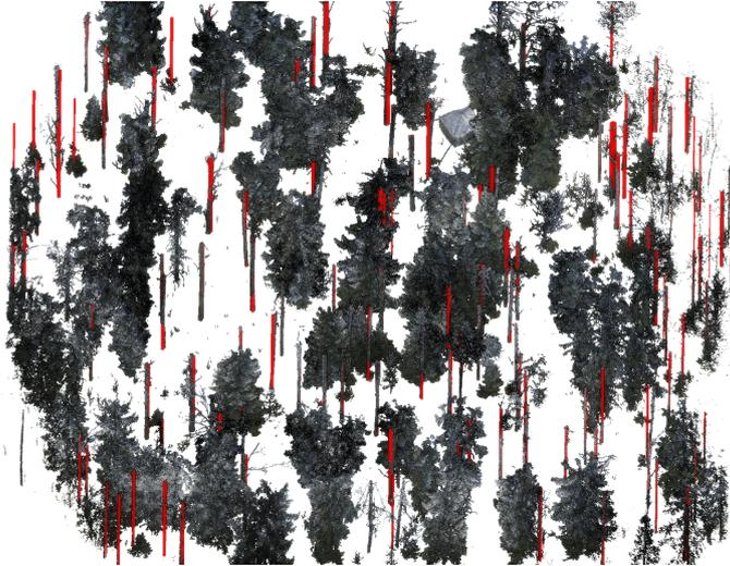
Figure 4: Qualitative results of our cylinder fitting approach, where fitted cylinders are shown in red. The point cloud has been cropped along its height to allow a better visualization.
