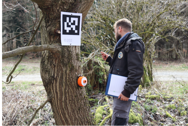
Figure 4: For association of reference measurements by forestry experts and trees in the forest recorded by our sensors, we used AprilTags [20] to identify the trees automatically in the recorded data and correlate this with recorded measurements.
